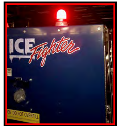
Steady Red Indicates Low Fuel Red Flashing Indicates an alarm state (Heater Lockout) Fast Flash rate is selectable at 80/min. or 240/min.
