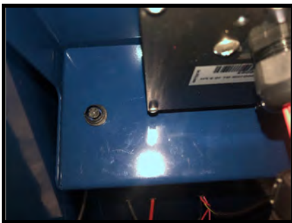
Connector Mounted On Rear of Main Control Panel Permits Fast And Simple Connection Of Beacon
