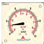
Typical manifold pressure reading high-fire NATURAL GAS
