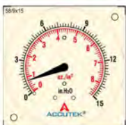
Typical manifold pressure reading high-fire PROPANE
