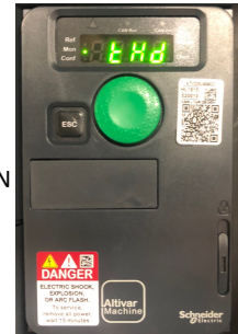
DRIVE THERMAL STATE 100%=NORMAL 118%=OHF THRESHOLD
