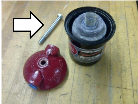
Figure 1: Center bolt removed from filter
