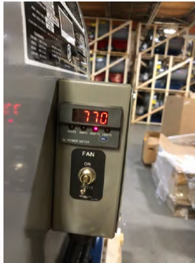
Meter showing the watts being used by the heater
